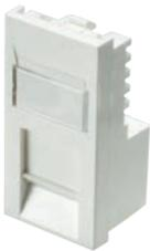
Excel Category 5e RJ45 modules comply with the EIA TIA Standard for enhanced Category 5. Each shuttered module is supplied with a slide label field and space above, this is allowed for use of self adhesive or further labelling if required. Termination can be made using Krone tooling, a cable tie base is positioned to the side of the IDC blocks to relieve cable stress.
