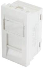
Excel Category 5e RJ45 modules comply with the standard for enhanced Category 5. Each shuttered module is supplied with a slide label field and space above, this is allowed for use of self adhesive or further labelling if required. Termination can be made using Krone tooling, a cable tie base is positioned between the IDC blocks to relieve cable stress.
