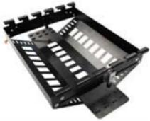
The Excel 24 port overhead tray consolidation point has been designed to allow 24 LJ6C modules to be installed onto standard basket tray allowing up to 24 connections to be installed above cabinets or anywhere along the containment run where extra points are needed. The unique locking mechanism allows the unit to be fitted / moved easily. The frame hooks onto the basket tray and the two push button plungers hold the frame in position.
