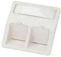
The Excel Angled 2 Port Keystone 50 x 50 mm Faceplate comprises of the fascia and mounting frame in an option of colours. The frame accepts all of the Unscreened and Screened Excel Keystone Jacks and presents them in an angled orientation to reduce the depth of the back box. The mounting frame is complete with a fitting to accept a 6mm spade connector if earth bonding is required.
