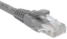
Excel Category 6<sub>A</sub> U/UTP patch leads consist of 4 twisted pairs of 26AWG stranded copper wires. These pairs are then cabled together, with different lay lengths to ensure optimum performance. Staggered pin RJ45 plugs, terminate the cable, and each lead is fitted with colour coded slimline moulded boots, suitable for use in high density router or switch blades.
